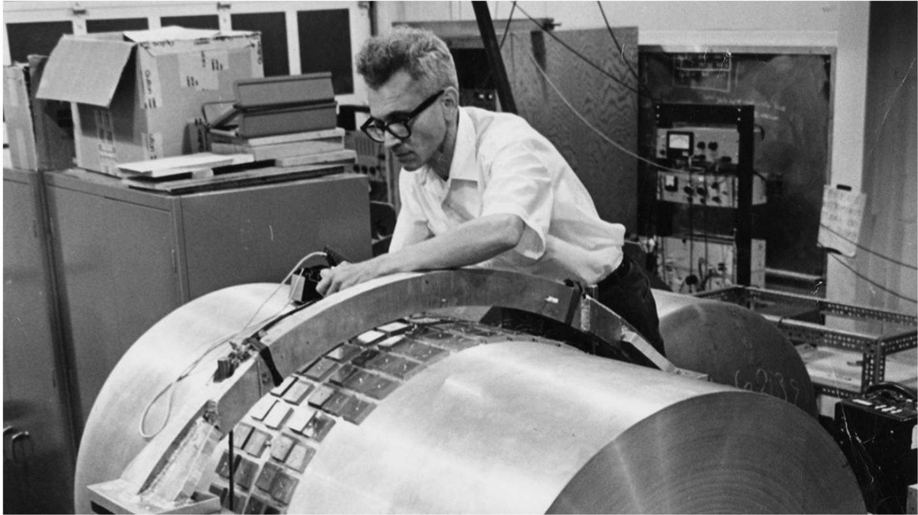
Joseph Weber and one of his gravitational wave detectors. SPECIAL COLLECTIONS AND UNIVERSITY ARCHIVES, UNIVERSITY OF MARYLAND LIBRARIES
